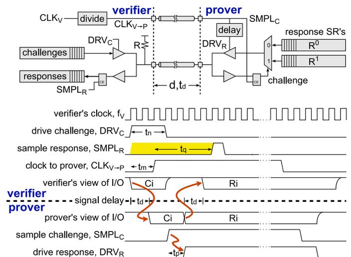
The distance resolution we can achieve is defined by the operating frequency of the verifier and so should have a fast clock, whereas the prover can operate at low frequencies and use delay lines to derive critical signals. **We have tested the system with various transmission lengths and confirmed that it is indeed able to detect small additions to the signal transmission distance.**
